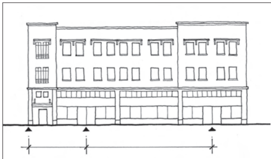
Figure 3.C.64: Table 3.C.1 provides Guidelines that allow flexibility in the location of entrances for various types of uses.
