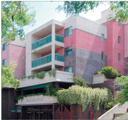
Figure 3.A.21: (Example of Poor Design) Color changes alone do not create attractive building façades. Articulation and architectural detailing should also be incorporated.
