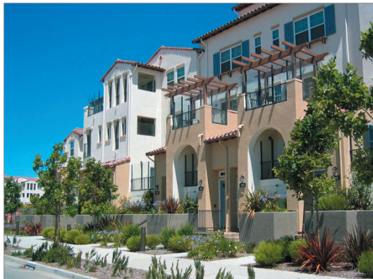
Figure 3.B.42: Use of Bays, Decks, and Trellises to Create Façade Variation and a Human-Scale
