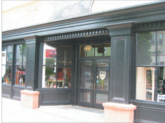
Figure 3.C.65: Recessed building entries commonly found in Vallejo's Downtown provide display or seating space as well as clear space for pedestrians along sidewalks.
